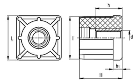
$\begin{array}{lll} d & = M8 \\ h & = 10 \\ H & = 31 \\ h1 & = 6 \\ Internal tube size = 26.0 \\ I & = 26.0 \\ L & = 30 \\ \end{array}$
